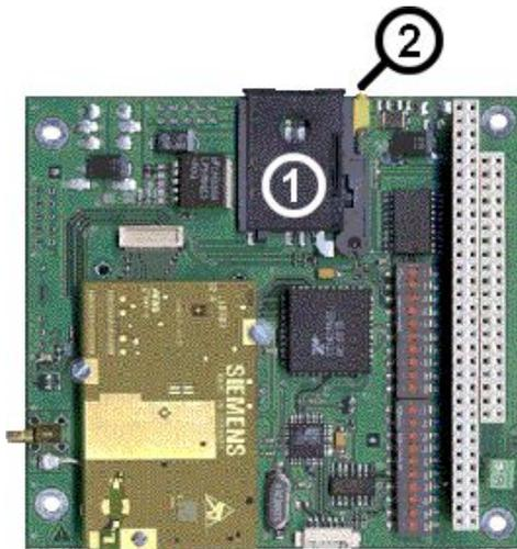
**Figure D.1:** Mounting a SIM card on the modem circuit board
