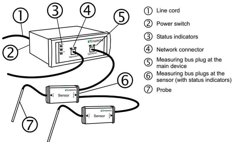
**Figure 2.1:** Connecting the main device and the sensors
